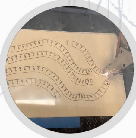
Puzzle structure model making using laser cutting
