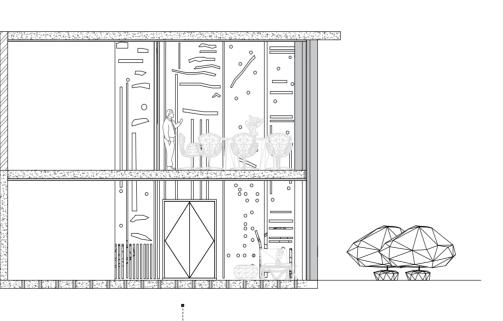
The decorative wall ( 250 mm)-entrance is made of bioconcrete and the decorations with clear triple glass
