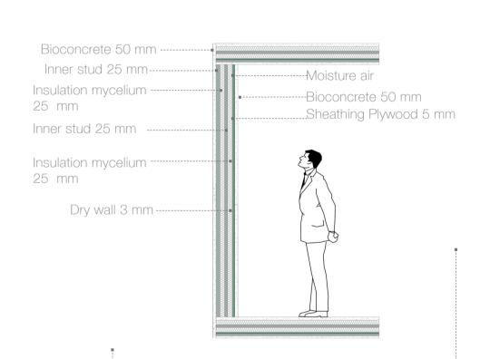
Details thermal insulation pasisve building office The skin of the building – walls, windows, and the roof – moderates the effect of the climate. Selection of building envelope with appropriate thermal mass, insulation, and color based on climate and functional requirements can reduce the number of hours when heating or cooling is required to maintain comfort.
