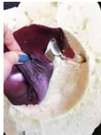
pull balloon plastic away slowly from expanding foam walls
