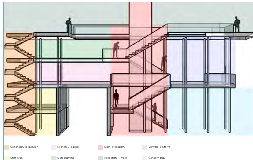
Figure 34 Diagram displaying zones within the building and visual connection between floors (Burford, 2023)
