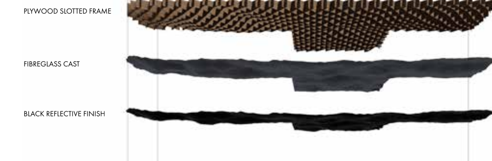
Rendered diagram demonstrating how the ceiling can be built with 1m x 1m squares of prefabricated fibreglass.
