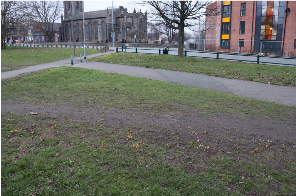
Fig 7. Poor positioning of flora species forms man-made circulation routes emphasising the rejection of the dictated circulation.
