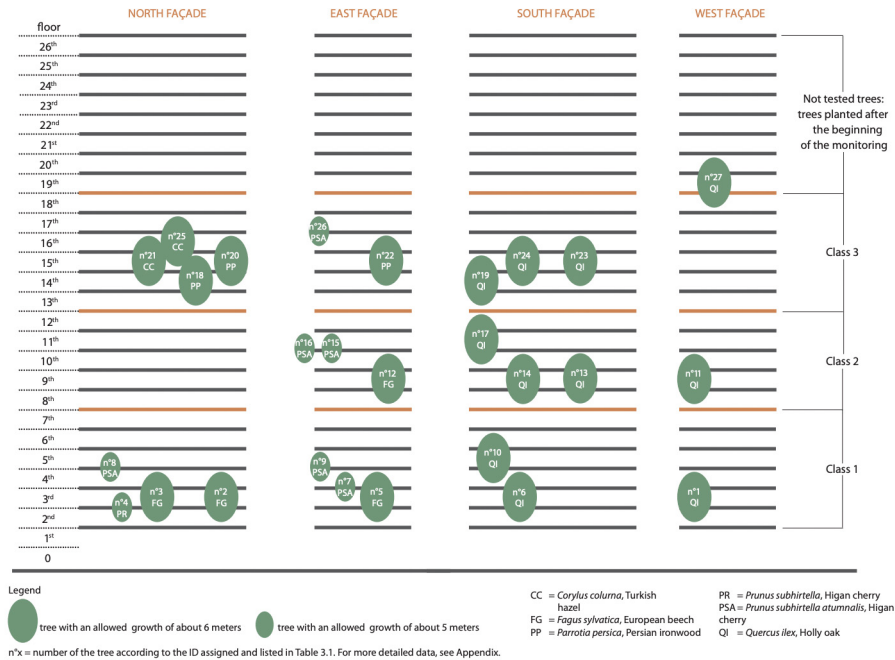
Fig 11. Diagram expressing the orientation of the tree plantations in relation to the north, east, south, and west facades of the building, whereby the long-term tests of the wind phenomenon and species selectivity enabled the position of the proposed areas of the site.
