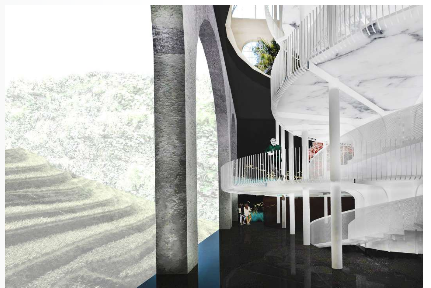
Rendered perspective showing the new exhibition entrance at the lowest underground level. Concrete arches support the original walls, mirroring the window structure above
