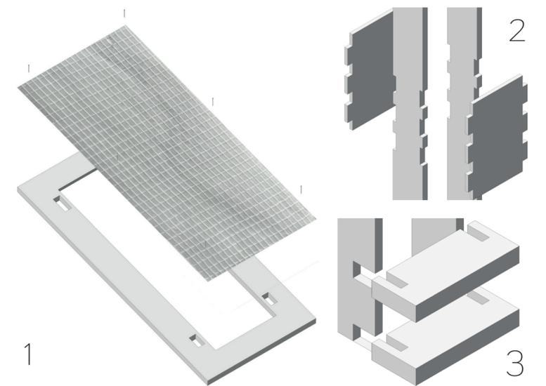
As we wanted to make sure the model is temporary and also can be easily built if needed at any point, the slotting method (2 & 3) was the most ideal building method. It is also used throughout the other areas of the pop-up show which brings some unity. The monarflex sheet (1) would be nailed into the roof framing to make sure that the artwork would stay dry in case of bad weather.
