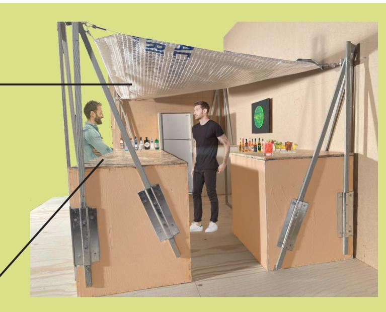
Inbetween the IBC tanks, will be metal box frames with OSB panels inlaid into them. OSB will also be used as tops for all structures.
