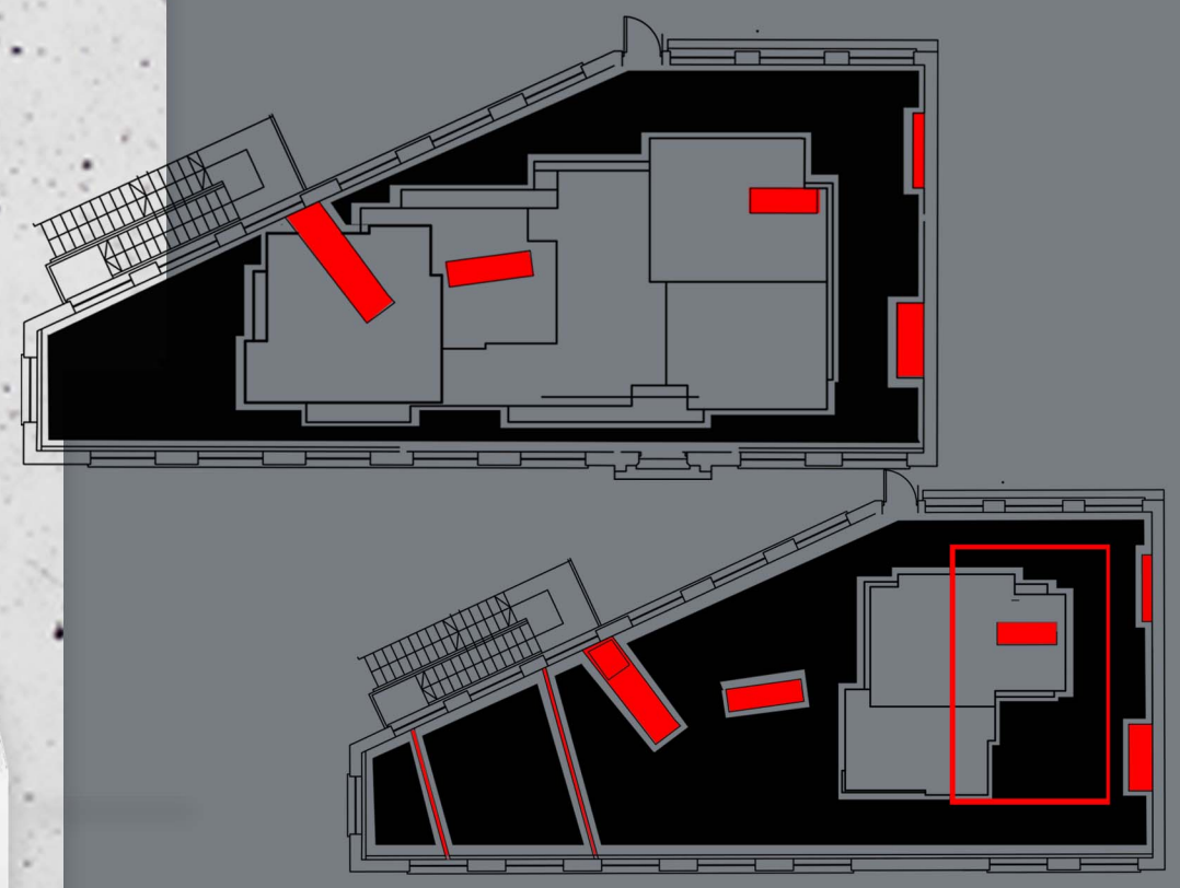
Forming Voids And Cut Outs Around The New Facade.
