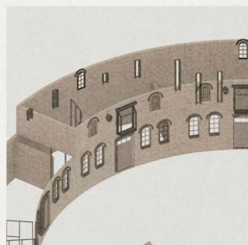
IMPROVING BUILDING'S ENERGY EFFICIENCY - new windows were built on South facade to introduce more natural light and connect the user with nature.
