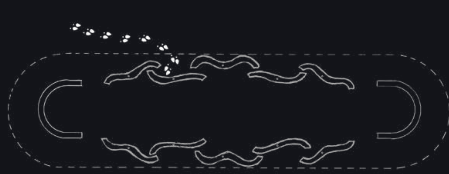
The pursuer is following and the person enters the structure at one of the cuves pushing the segments which then knock into the other segments on that side of the shelter
