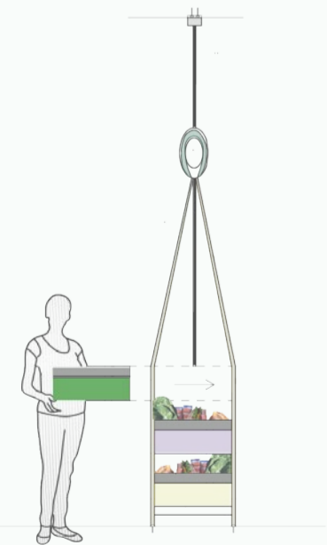
3. Here all the boxes have moved down to the bottom, so the new empty box (from which the food is taken to the prep room) is replaced on the conveyor ready to be filled up again.
