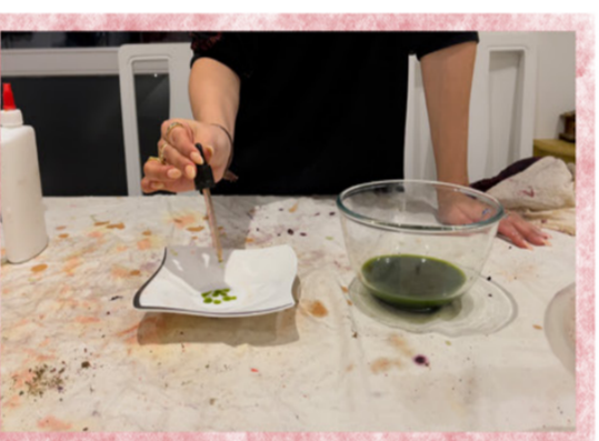
The pigment is tested with 4 different binders: liquid acrylic, PVA, egg yolk and gum arabic. The pigment is carefully added to each binder. Using a pipette and mixed in gradually to test how much pigment is needed for each binder.
