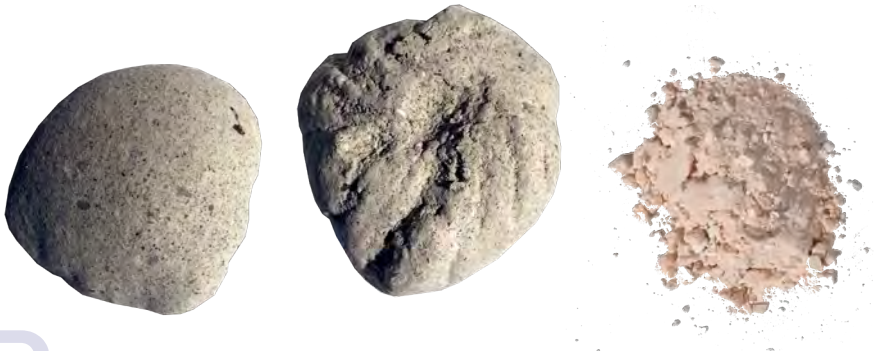
Above: cast slipper-crete. Right: Powder lime made from slipper limpets with the addition of brick dust.
