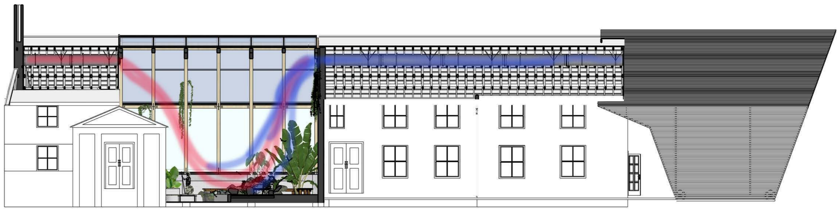
ducting controlled temperature air in roof space.
