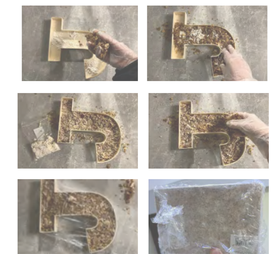
Testing the efficiency of curved moulds for mycelium growth
