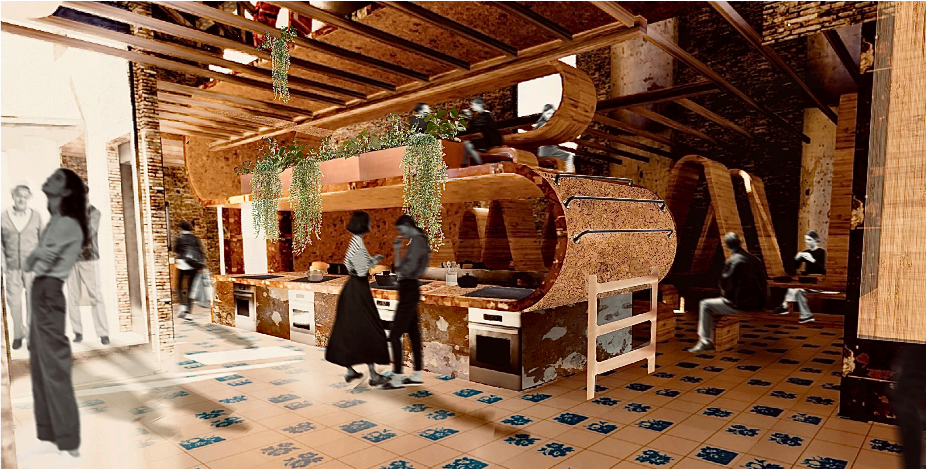
3D Visualisation depicting the use of the linocut tiles, the wallpaper roll (replicating the previous wallpaper), the exposed beams and joists and the cork structures. The chimney breasts which as scattered with holes have not been plastered and will remain the same to leave a sense of the spaces history.
