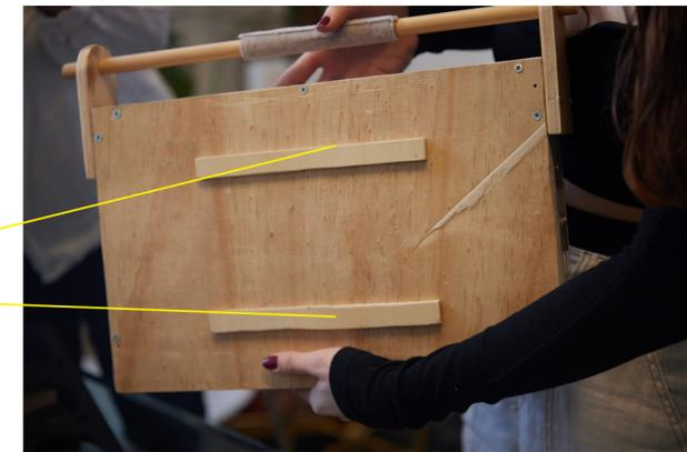
Two pieces of wood that allows the attached platform to stay stable when moved
