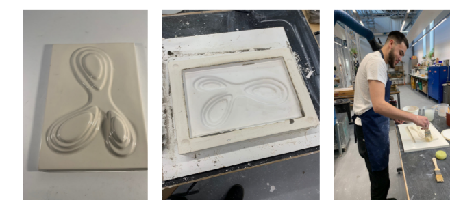
Bespoke tile making for basement
