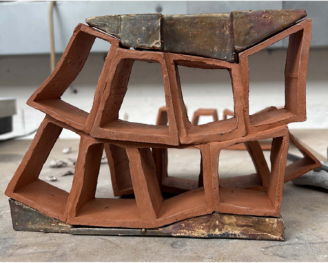
Lost wax casting the wax areas to transform into Bronze.
