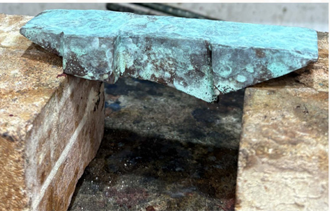
Adding layers of verdigris (green/blue) & liver of sulphur (orange/red) patinas.
