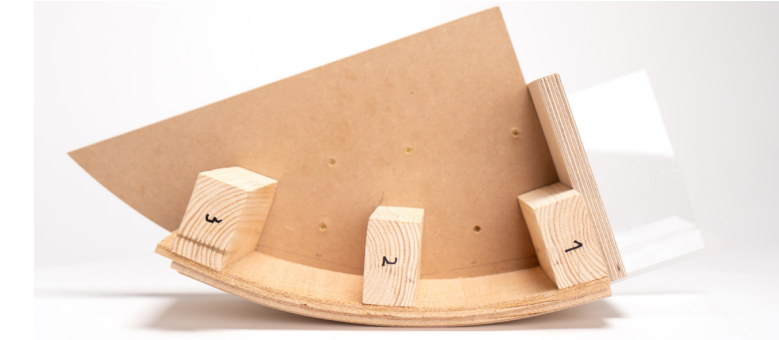
1:1 detail structural detail of bar X cake cabinet (curved birch ply front)
