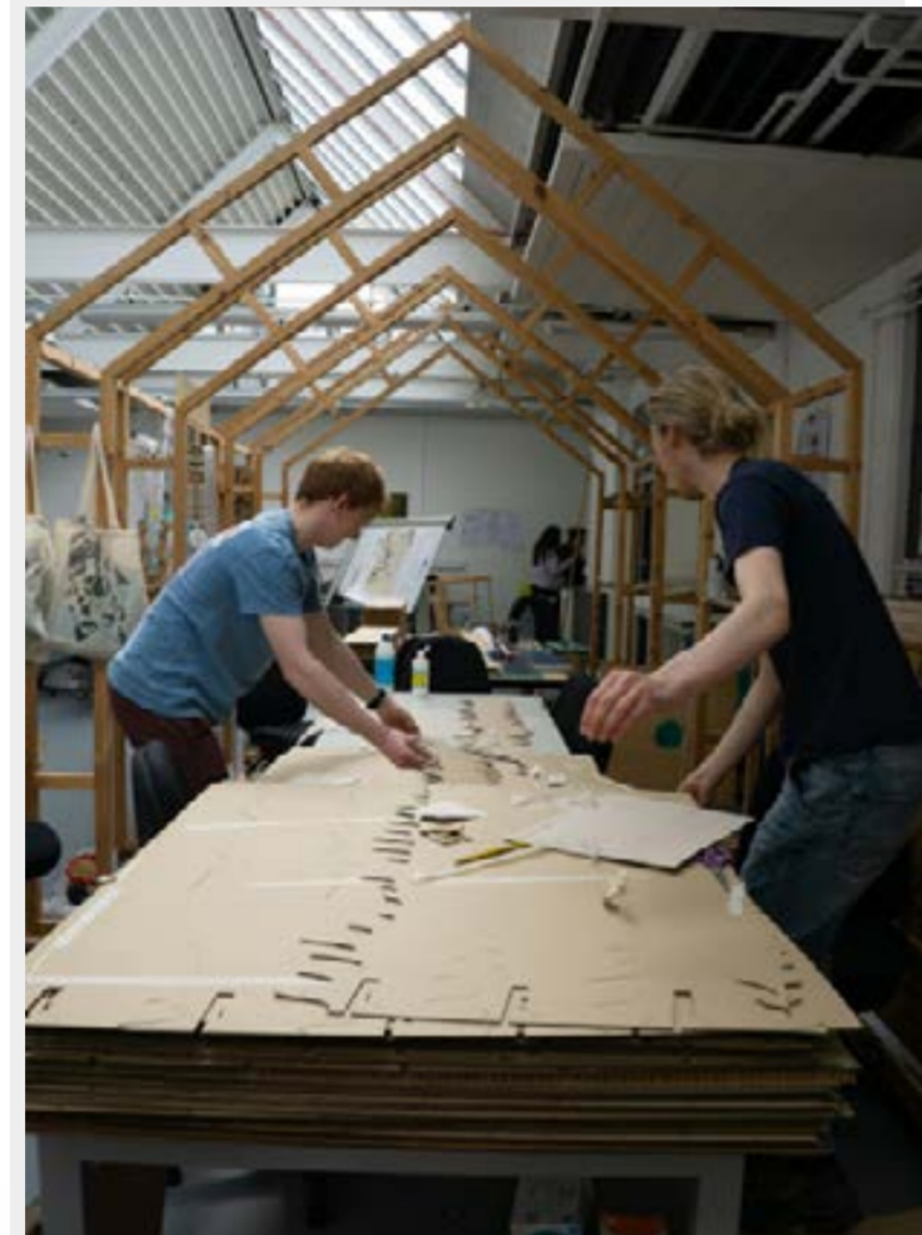
The pattern was scaled to the exact proportion of cardboard panels to create as little wastage as possible.
