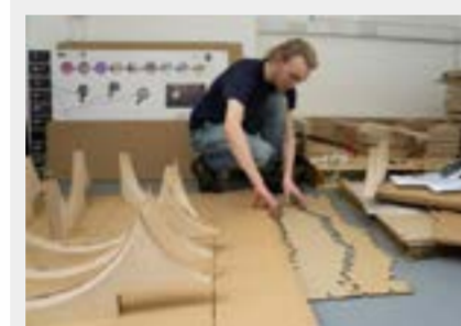
To use the pattern continuously, the sections needed to be offset so that there would always be a full strip to support where lines intersected.
