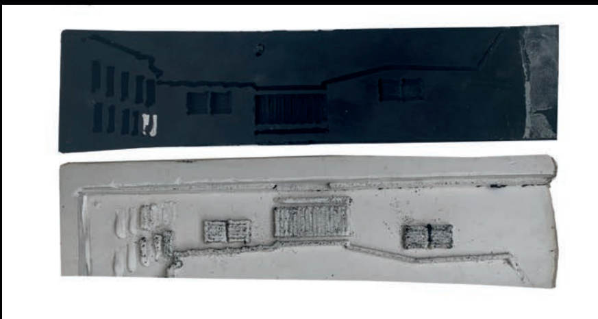
CNC Rubber Mould and Plaster Cast
