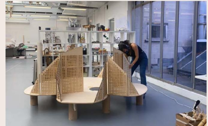
The geodesic dome was then assembled starting from the centre. I quickly found that the weight had to be supported during construction otherwise tension was put on the dowel plugs. This meant one broke.
