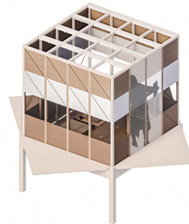
5. MAGNETISED PANELS INSERTED BETWEEN POSTS 25 minutes
