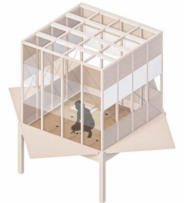
6. FLOOR MATTING PANELS LAID 10 minutes
