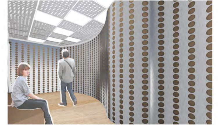
Interior clad with perforated metal with foam backing.
