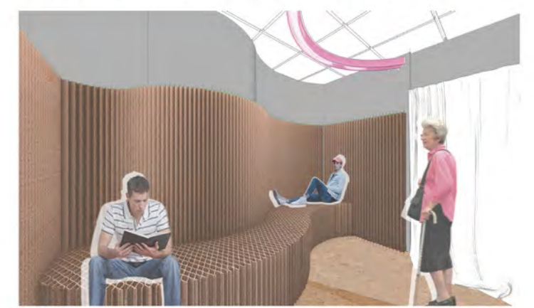
Rubber Cork flooring and Nonwoven Polyethylene seating and acoustic ceiling tiles, to maximise sound absorption.
