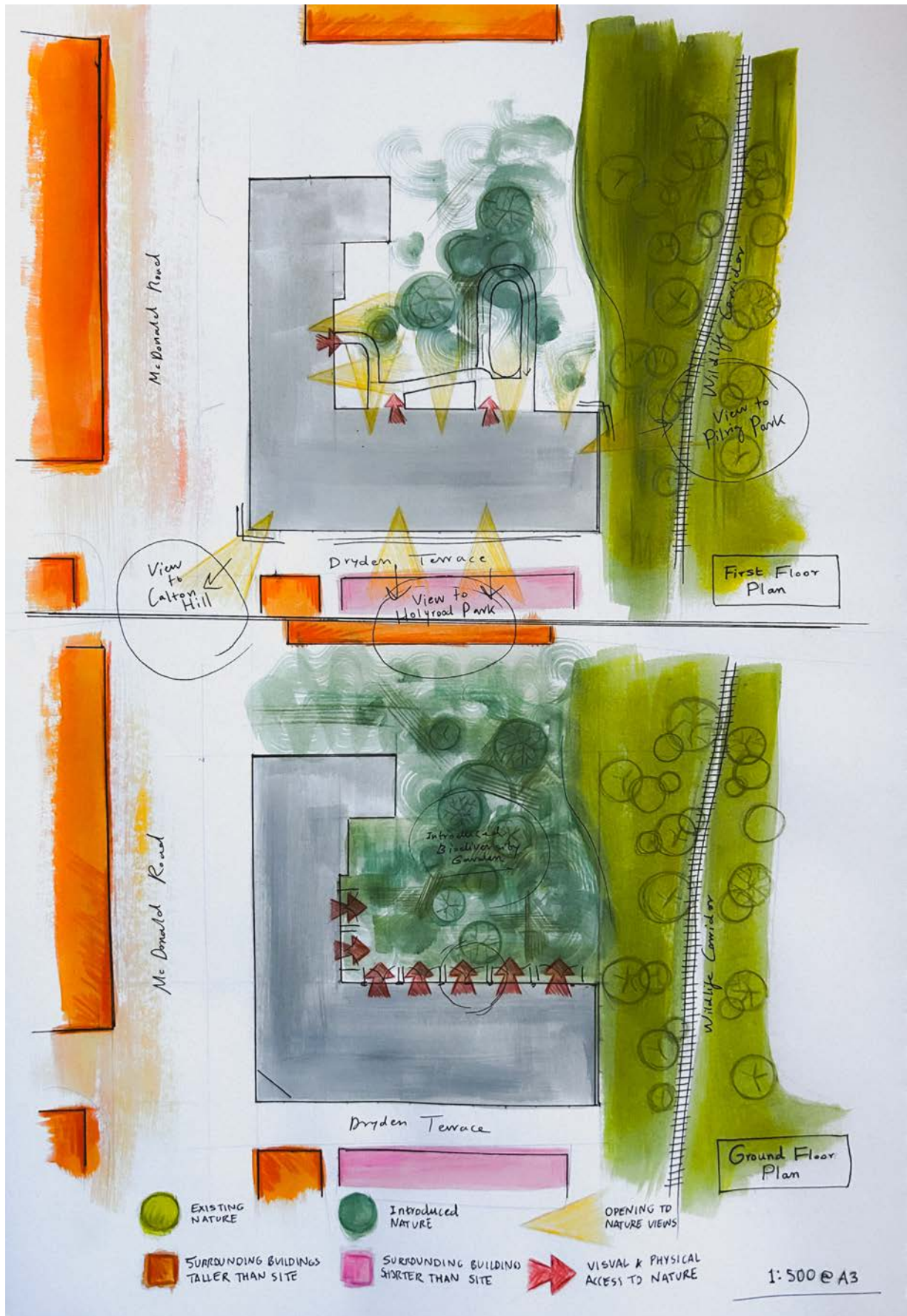
Fig 3.1 - Configuration of Openings, ground and first floor plans. This illustration explores the building's possibilities to offer visual and physical access to the garden and views to surrounding nature.
