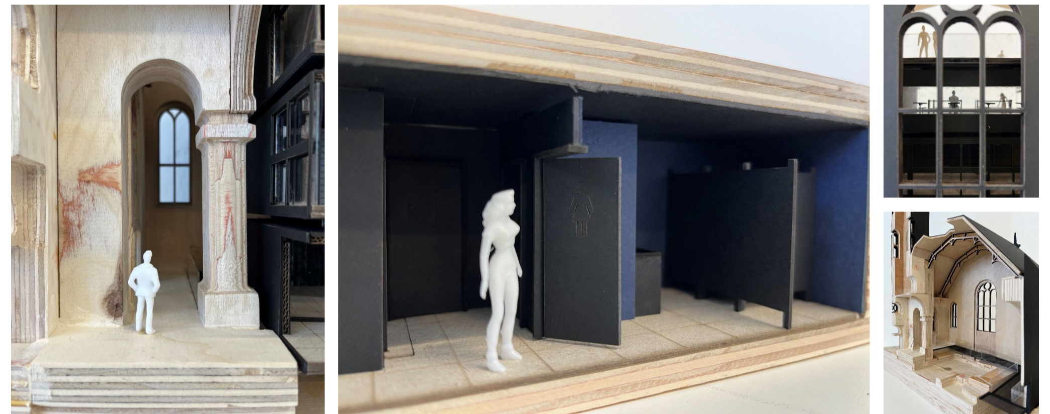
1:50 sectional model made of plywood and black card. The plywood is representative of the historic stonework still on display at the site. The black card represents the new independent structure of the library in the interior. The two materials display a contrast between the traditional building shell and the contemporary interior intervention, as well as a harmony between the two layers.
