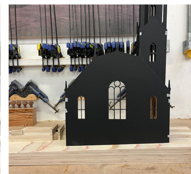
To translate the design into a physical model, I chose to use plywood and the CNC machine for the exterior and existing walls of the Tron Kirk. From this, the details and character of the brickwork and archaeology below are most represented. The outside of the model is clad in black card with minimal exterior details to draw focus onto the interior of the model, and loosely reflect the dark nature of the exterior of the Tron Kirk.
