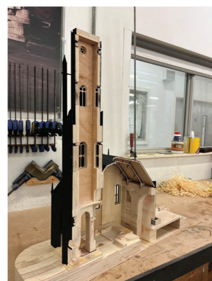
To translate the design into a physical model, I chose to use plywood and the CNC machine for the exterior and existing walls of the Tron Kirk. From this, the details and character of the brickwork and archaeology below are most represented. The outside of the model is clad in black card with minimal exterior details to draw focus onto the interior of the model, and loosely reflect the dark nature of the exterior of the Tron Kirk.
