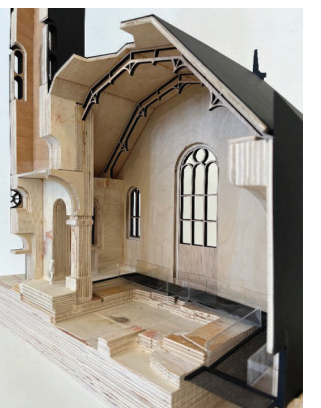
1:50 sectional model made of plywood and black card. The plywood is representative of the historic stonework still on display at the site. The black card represents the new independent structure of the library in the interior. The two materials display a contrast between the traditional building shell and the contemporary interior intervention, as well as a harmony between the two layers.
