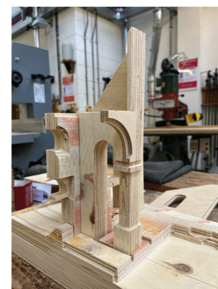
To translate the design into a physical model, I chose to use plywood and the CNC machine for the exterior and existing walls of the Tron Kirk. From this, the details and character of the brickwork and archaeology below are most represented. The outside of the model is clad in black card with minimal exterior details to draw focus onto the interior of the model, and loosely reflect the dark nature of the exterior of the Tron Kirk.
