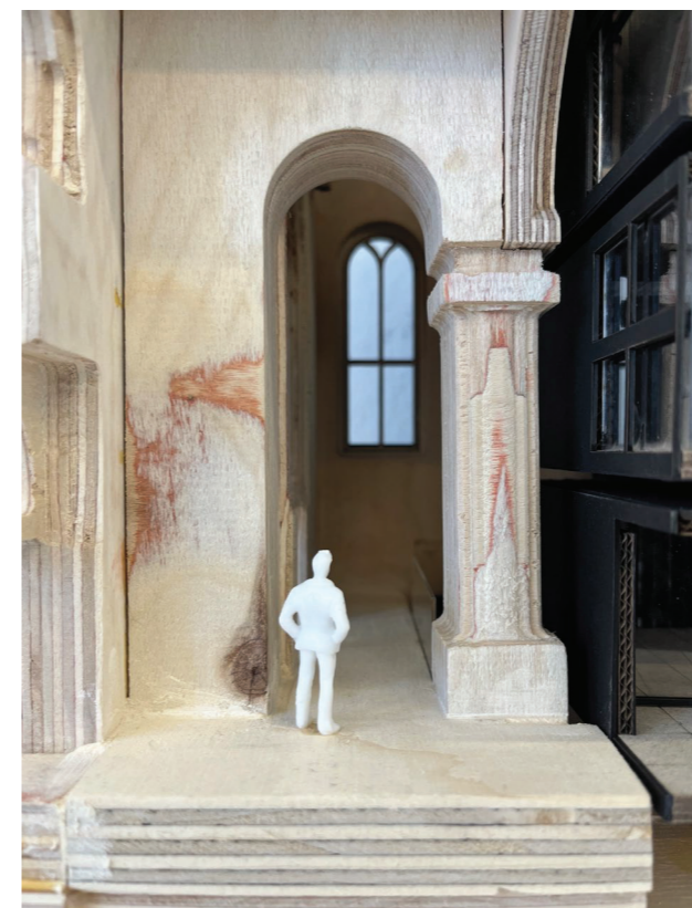
1:50 sectional model made of plywood and black card. The plywood is representative of the historic stonework still on display at the site. The black card represents the new independent structure of the library in the interior. The two materials display a contrast between the traditional building shell and the contemporary interior intervention, as well as a harmony between the two layers.
