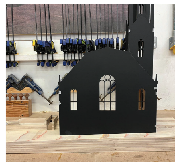
To translate the design into a physical model, I chose to use plywood and the CNC machine for the exterior and existing walls of the Tron Kirk. From this, the details and character of the brickwork and archaeology below are most represented. The outside of the model is clad in black card with minimal exterior details to draw focus onto the interior of the model, and loosely reflect the dark nature of the exterior of the Tron Kirk.
