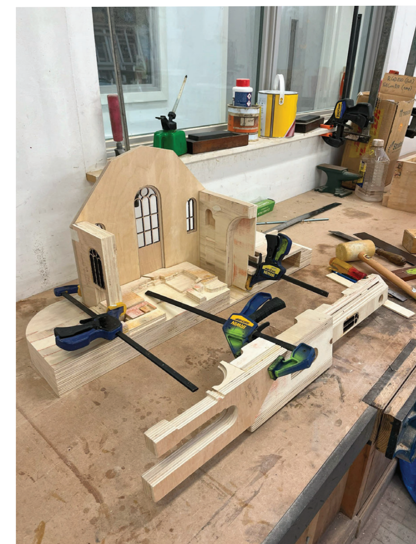
To translate the design into a physical model, I chose to use plywood and the CNC machine for the exterior and existing walls of the Tron Kirk. From this, the details and character of the brickwork and archaeology below are most represented. The outside of the model is clad in black card with minimal exterior details to draw focus onto the interior of the model, and loosely reflect the dark nature of the exterior of the Tron Kirk.
