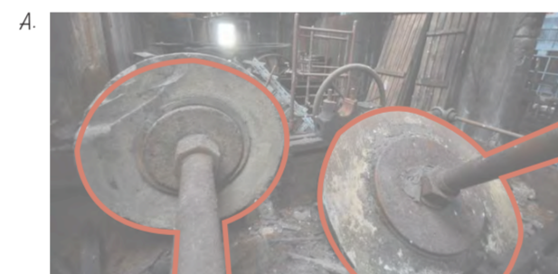
Flywheels? Store kinetic energy. In the Industrial period were usually made with heavy rims made out of cast iron. They were utilised to dampen the pulsation in engines, machinery, etc.
