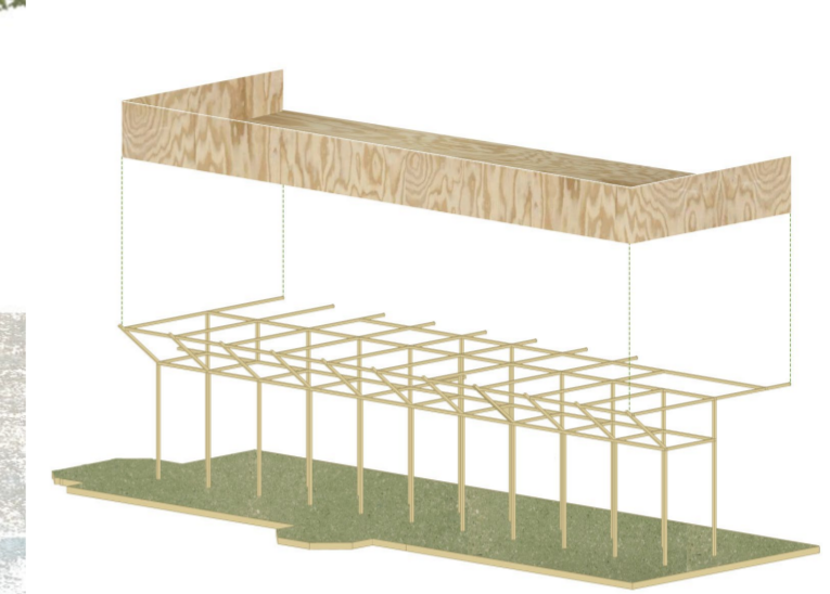
02 Support of the First Floor
