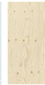
**Cross-laminated timber (CLT)** is the main material for its sustainable qualities, but for its aesthetic as well. CLT is a wood panel product, made from gluing together layers of solid-sawn lumber. CLT is easy to mold in shape and it is possible to recycle as well.
