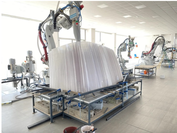
Fig.26: Hassell Studio and NAGAMI (2020) 3D printing of the pavilion [photograph], Hassell Studio and NAGAMI, Avila, Spain
