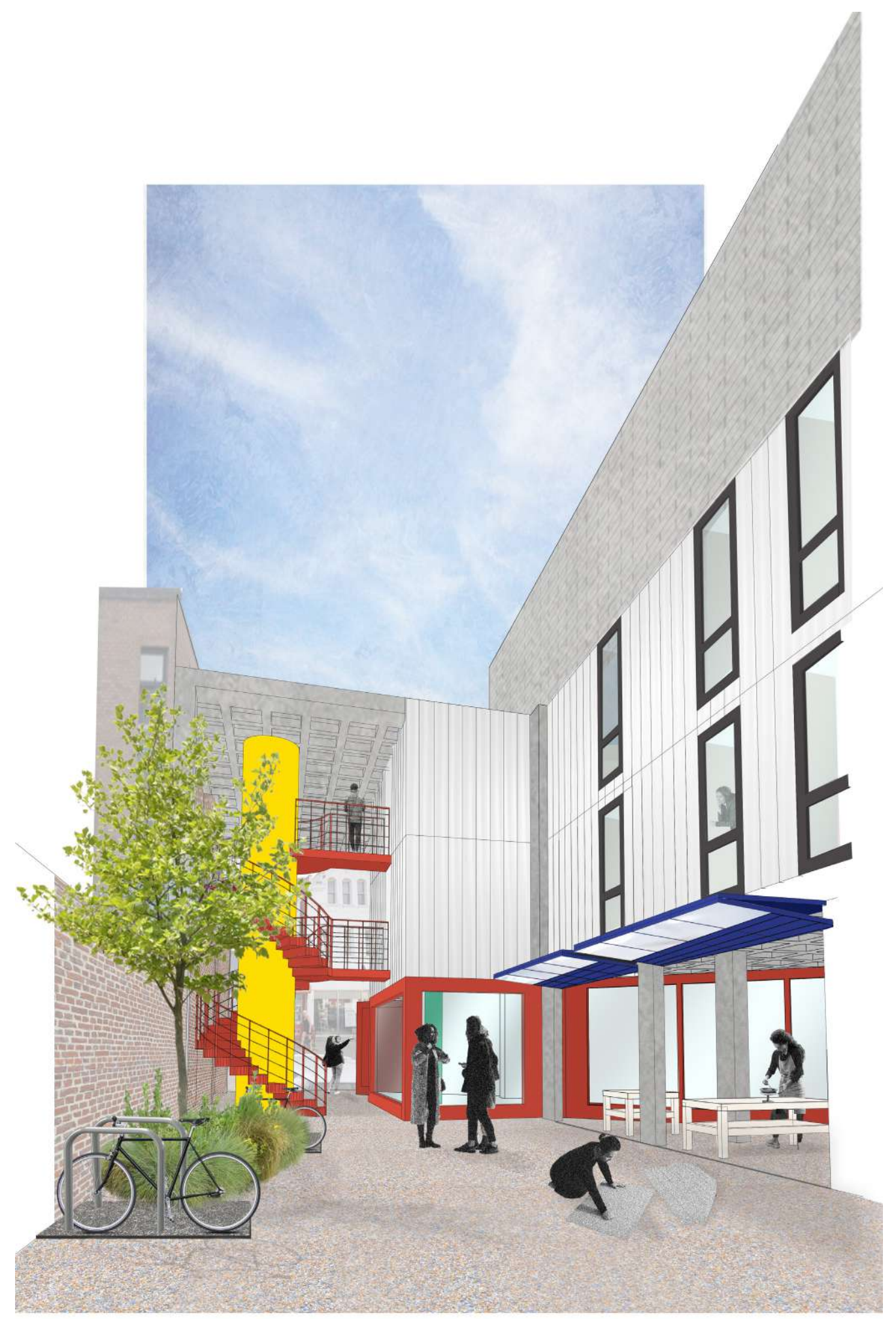
View from courtyard with 3D workshop garage doors, channel glass first and second floor facade, external staircase and plant room.
