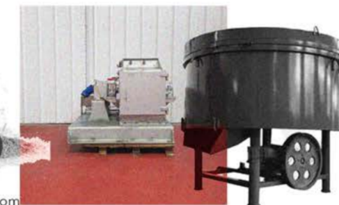
Decorticator Used to separate the outer fibers (bast fibers) from the inner woody core (hurd) of the hemp stalk.
