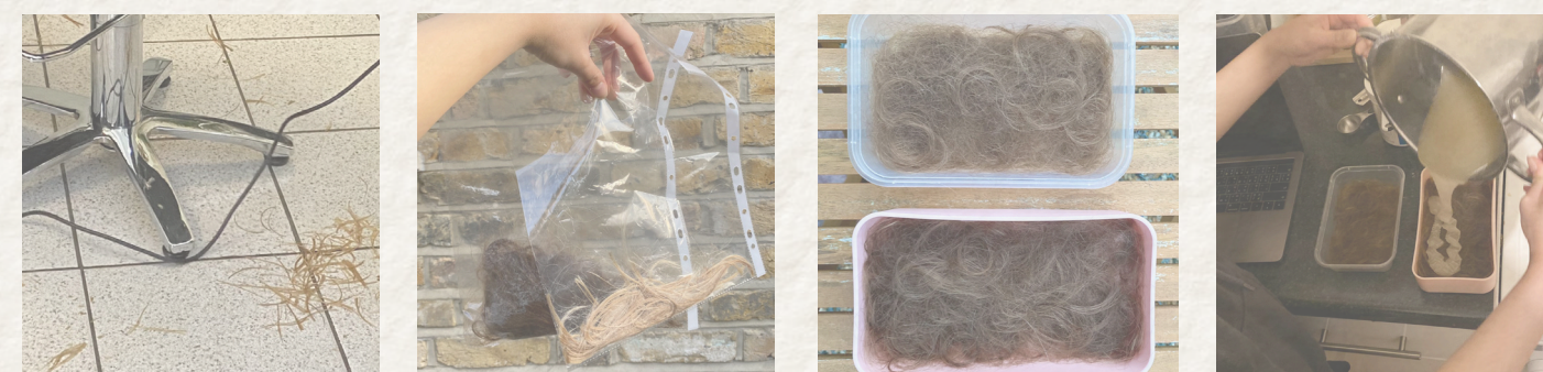
1. Hair collected from the salon 2. Hair washed and sorted 3. Hair placed in the molds 4. Bioplastic paste poured on top
