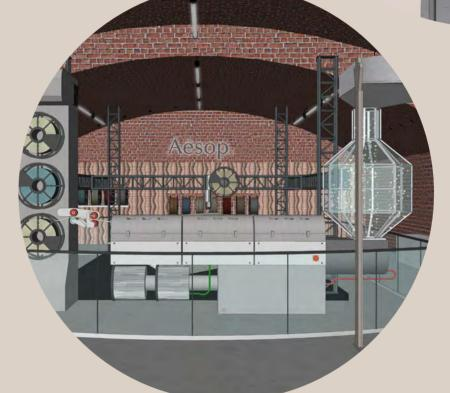
5. The shredded plastic then enterers the next machine that heats the plastic and transforms it into 3D printing filament.
