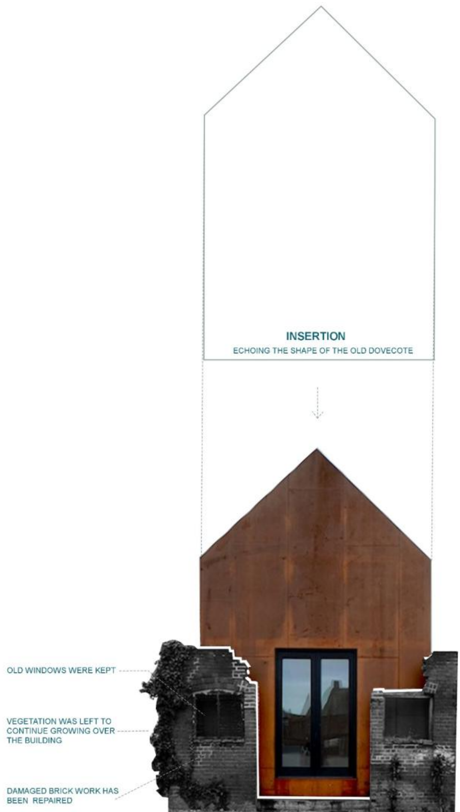
FIGURE 38: DOVECOTE STUDIO RENOVATION PROCESS DIAGRAM (RABIJ, 2021) ORIGINAL SOURCE (VILE, 2010)
