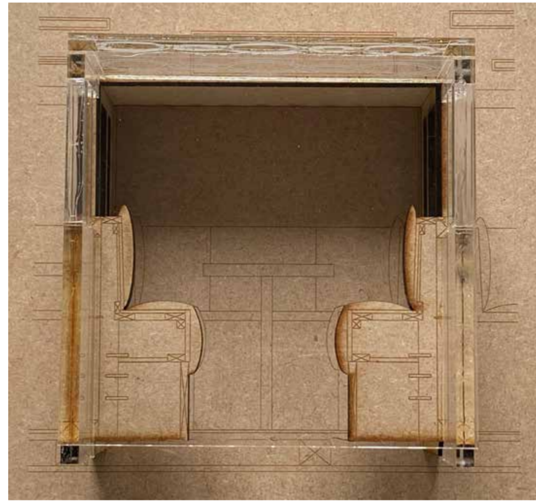
Hybrid Detail Model of the booths in section using MDF and acrylic
