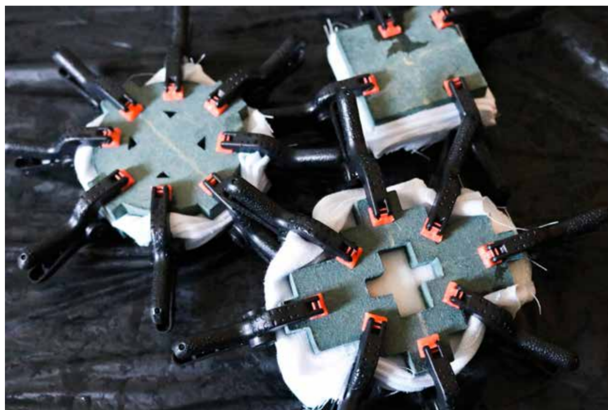
Method: binding the wooden blocks and folded fabric with clamps.
