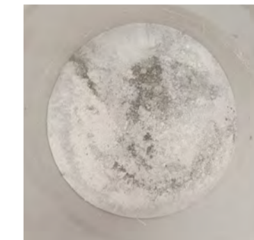
[dry mix - lime + cement + water]
