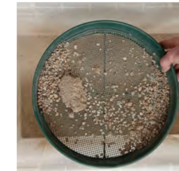
[sieve the demolition debris]
