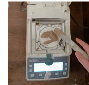
[test moisture level of the sand]
