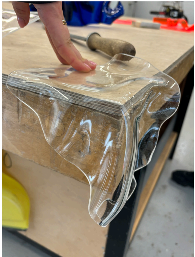
Model testing in the wood workshop - melted waste acrylic.
