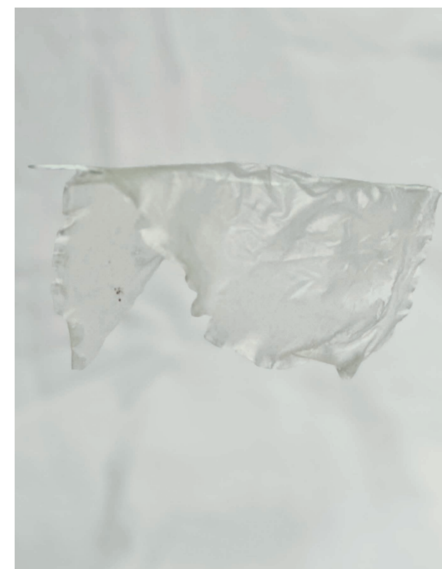
Bioplastic result. To make the material waterproof and increase its usage a coat of beeswax can be applied.
