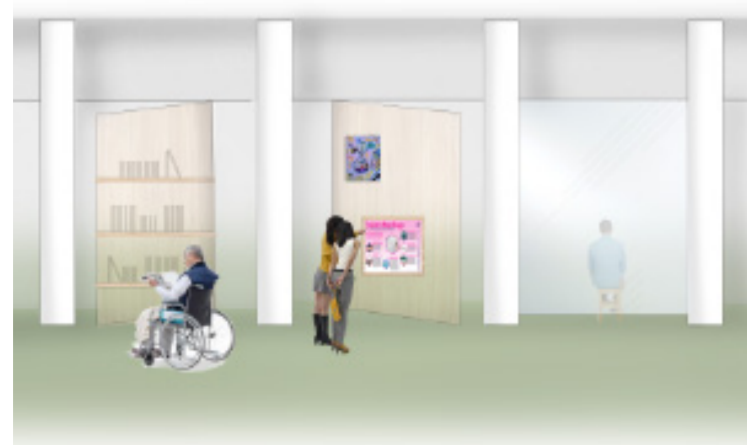
Pivoting bookshelves between the columns which can also close to allow for flexibility and privacy. Interactive.
