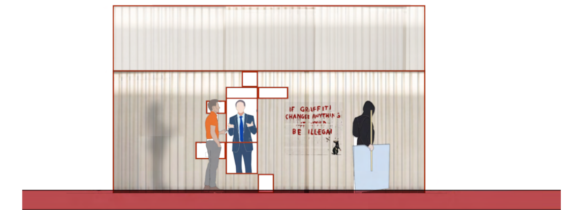
Town Hall is made out of glass channels to give them privacy while exposing their silhouettes. The windows are asymmetrical and provide a peek through into the spaces. The windows open for different functions for example asking a question
