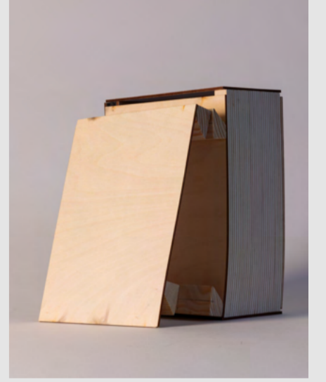
Plywood 1:1 sample. Batten allows for easy removal of the panels to be washed, reused and exhibition.
