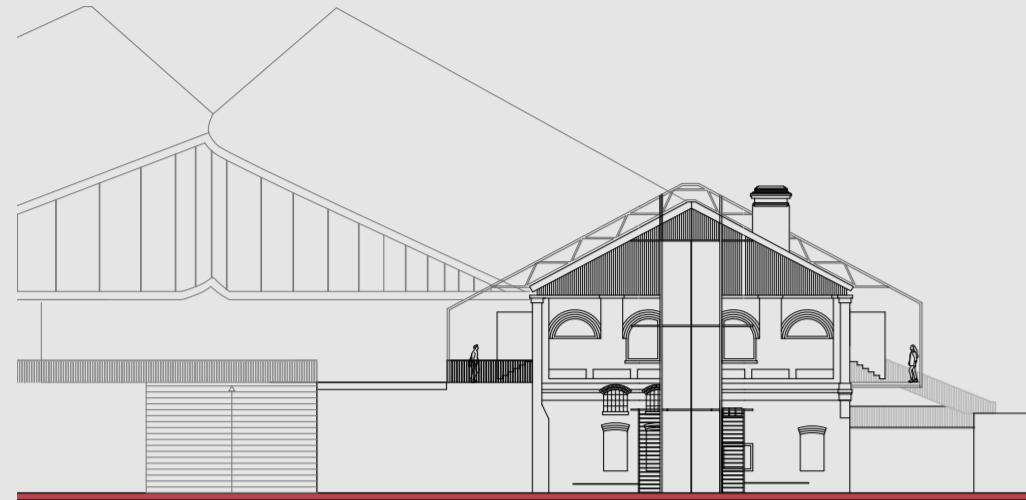
Front elevation showing corten steel, ladders and the slit.
