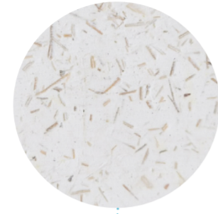
Lime hemp plaster
