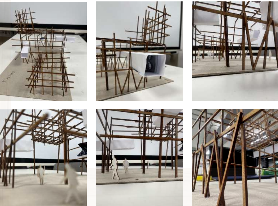
Maquette modelling. Looking at how the timber scaffold frame structure will work with the slotted in containers.
