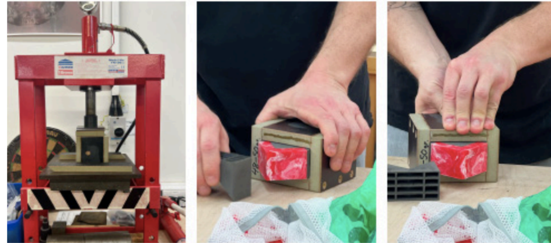
Taking the bracket out of the mould after waiting thirty minutes for it to cool down. This process was repeated seven more times as our two biggest correx box stands needed four each.
