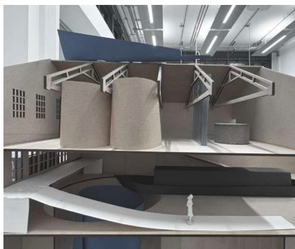
A ramp for easy access for visitors, while Preserving the historical barge. Shower rooms placed on the first floor. Water tank placed at beneath the ground level.
